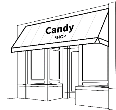
Figure 6-2: Awning and Canopy Sign
