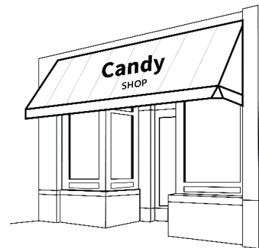
Figure 6-2: Awning and Canopy Sign
